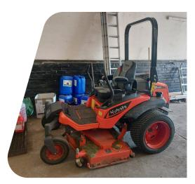
The new 'Kubota ZD turn mower' comes equipped with a mulching cutting system, and the results have been amazing. This system is designed to hold the grass clippings longer, cutting them into smaller pieces before putting them back onto the lawn. This feature offers several benefits that have now transformed how we cut your grass.
